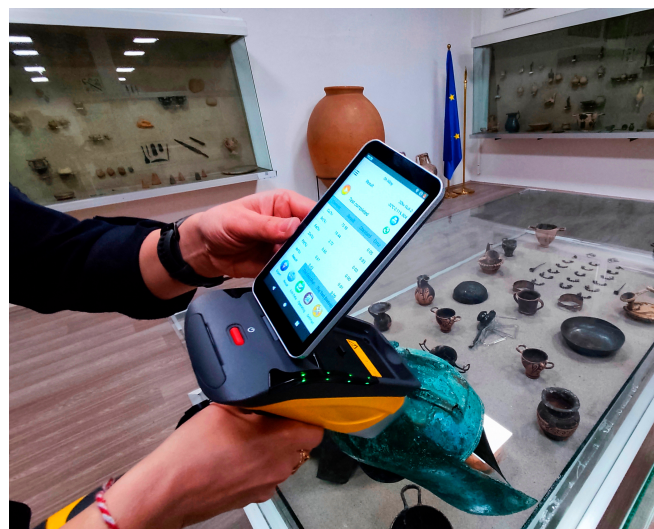
Figure 1. Explorer 5000 handheld XRF device (Skyray Instruments, Inc., Kunshan City, Jiangsu Province, China) while conducting measurements at the Institute of Archaeology (please see Supplementary Materials) (photo taken by the authors).
